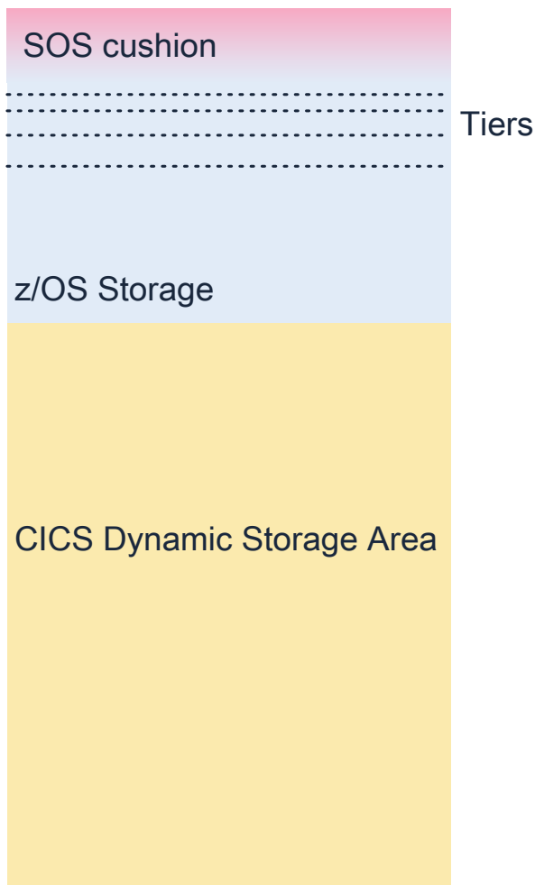
Figure 16. A schematic illustration of storage usage in CICS
